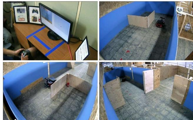
Fig. 1. To investigate whether a combination of audio and visual communication channels reduce workload and improve performance, we set up a test course and had a graphical interface (top left; also see Fig. 5) for robot operators to control a robot for a search and threat-defusal task (red block as threat, see bottom left). For this full run, please watch the accompanying video [6].
