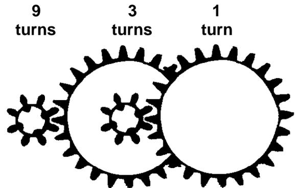
Figure 5: 9-to-1 Gear Reduction with Ganging
