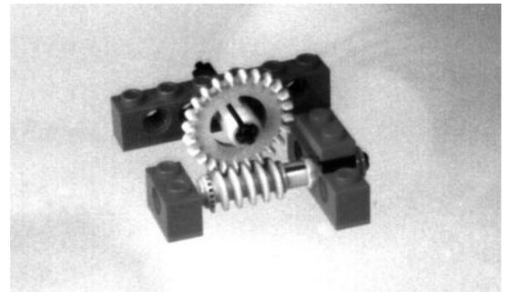
Figure 7: Using the Worm Gear
