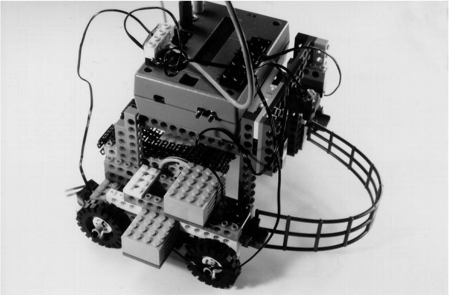
How many of the design clichés can you find in this robot? Look especially for the vertical spacing trick used to provide rigidity to the robot structure.
