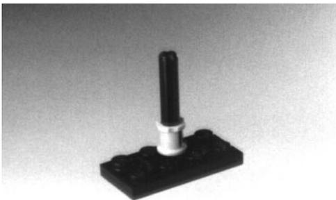
The full-size stop bush can be used in one orientation to hold an axle through a plate hole so that the axle can freely rotate. In Figure 24, an additional plate is used to trap the axle, but allow it to rotate freely.
