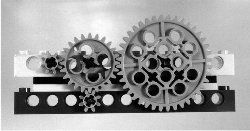
Figure 12: The Half-Radius Round Gears
