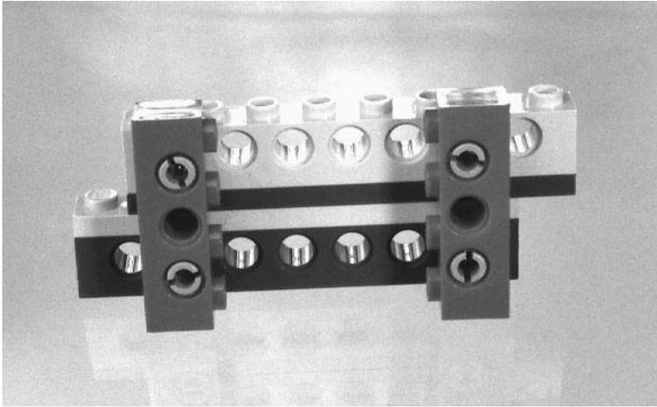
Two beams are separated by two  $\frac{1}{3}$ -height LEGO plates, creating a vertical interval of  $1\frac{2}{3}$  units, which is equal to 2 horizontal units. Hence the beams can be locked into place using cross-beams and connector pegs—the way to make your LEGO construction quite sturdy.
