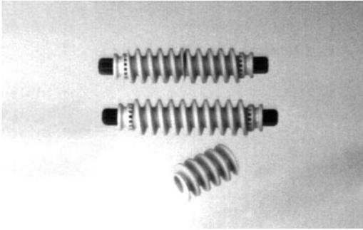
Figure 8: Multiple Worm Gears on One Shaft
