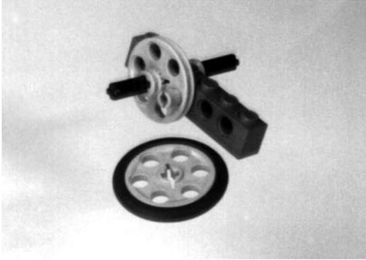
On occasion it is necessary to lock a beam to an axle. This figure shows how to use a medium pulley wheel, which rigidly locks to an axle, to hold the beam in place.
