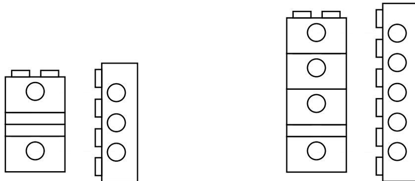
Figure 2: Creating Vertical Spacings with Two-Unit and Four-Unit Horizontal Measures
