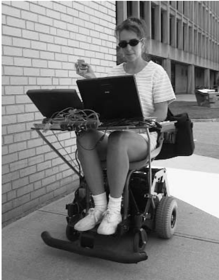
Figure 8-6: The robotic wheelchair system being driven with single switch scanning.
