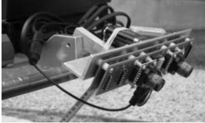
Figure 3-4: The Stereo Head mounted on the robotic wheelchair
