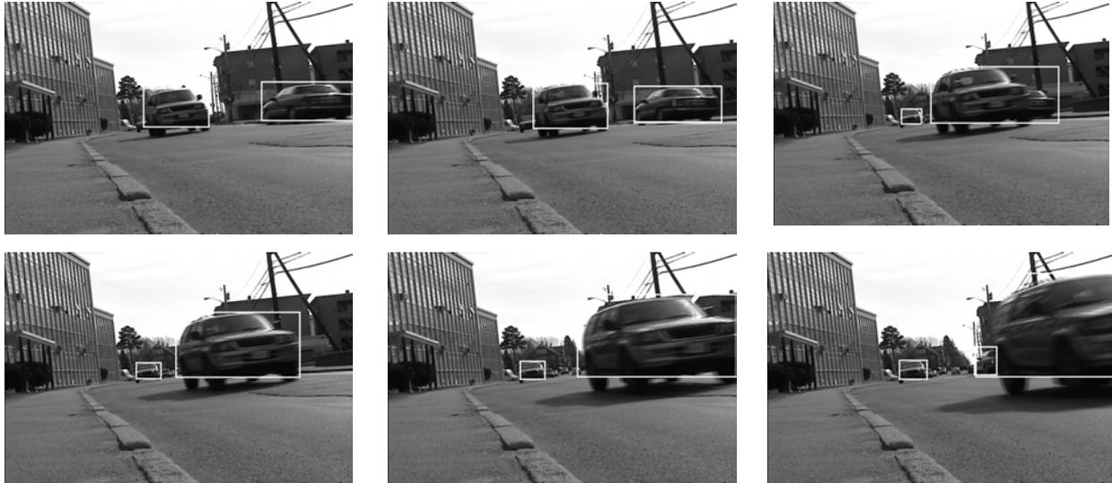
Figure 4. Six frames from a video sequence of approaching and passing vehicles from the robot's left-facing camera. The white boxes show the cars found by the tracking algorithm. The sequence shows the detection of a second approaching car as it gets closer. It also shows a passing car being tracked, then occluded by the oncoming vehicle, then finally tracked again as it emerges from behind the oncoming vehicle.
