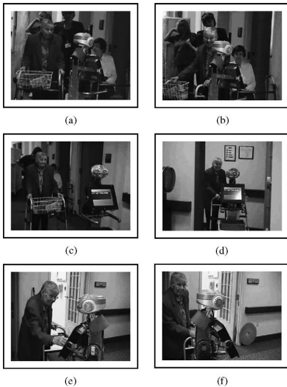
Fig. 7. Example of a successful guidance experiment: (a) Pearl picks up the patient outside her room; (b) reminds her of a physiotherapy appointment; (c) guides the person to the physiotherapy department; (d) enters the department; (e) satisfies a request for the weather report; (f) terminates the interaction and leaves.
