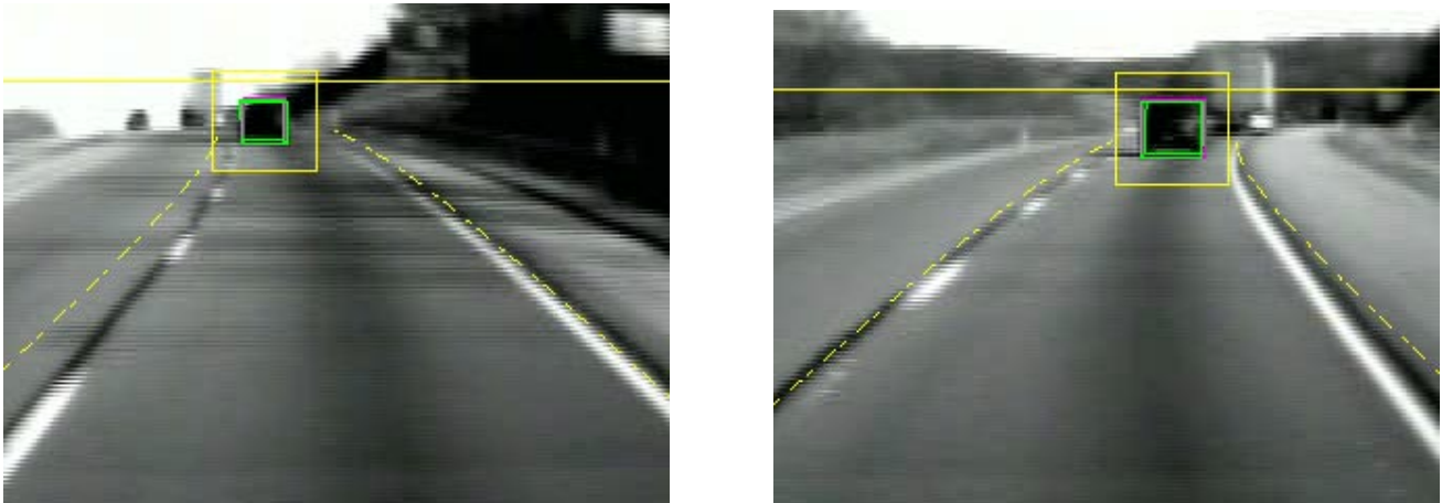
Figure 6. Two frames at t = 762 and t = 775 , both with large curvature and with the tracked vehicle clearly below the ground plane.
