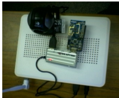
Figure 1: A SICS 802.11 wireless router with a Web camera and a 802.15.4 wireless sensor attached.
