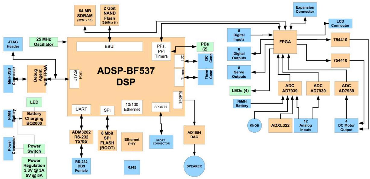
Figure 2: Block Diagram of the Blackfin Handy Board.
