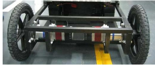
**Figure 4.2:** Vehicle Drive System
