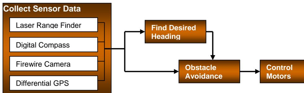
**Figure 6.2:** Software Structure for Both the Autonomous and Navigation Challenge
