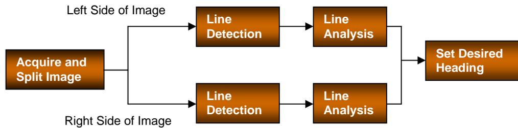
**Figure 6.3:** Flow Diagram of Autonomous Challenge Software
