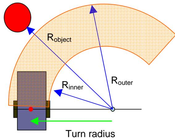
Figure 6.5: Distances used during obstacle avoidance
