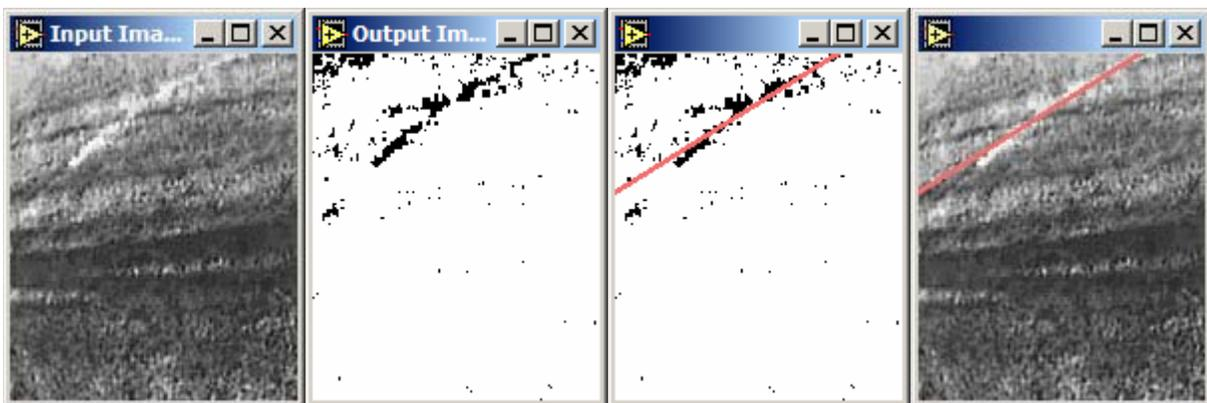
**Figure 6.4:** Original Image, After Threshold, Detected Line, and Original Image with Detected line
