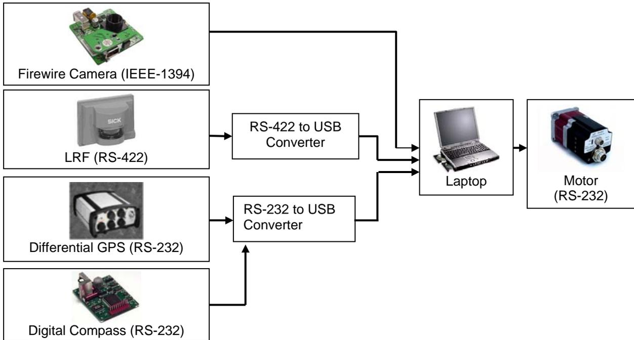
**Figure 5.2:** Component Communication Diagram
