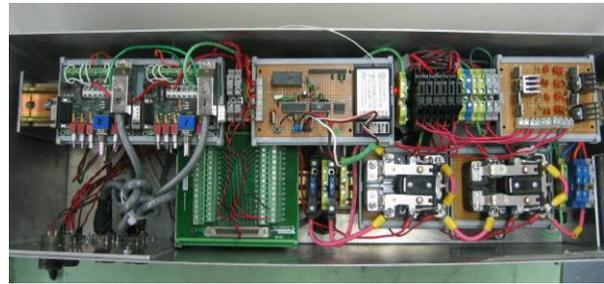
**Figure 5.1:** E-box Component Layout
