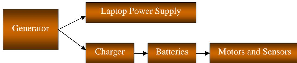
**Figure 3.2:** Block Diagram of Electrical System
