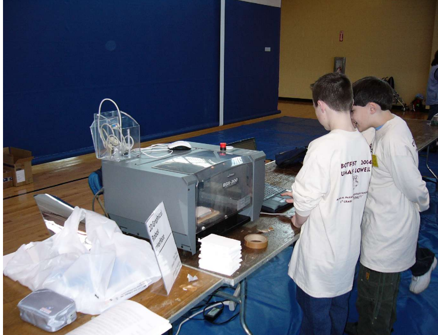
Figure3. The Roland engraving machine with white, foam-core poster board as the medium for output.
