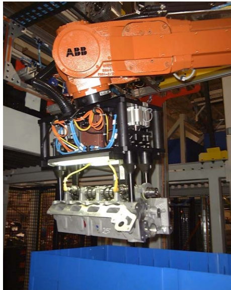
In this example, Braintech SC3D technology uses a single conventional CCD video camera to guide the robot to locate and then move an engine head from the conveyor and into dunnage.
