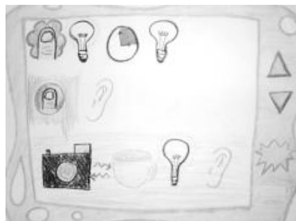
Figure 5: Some early visual programming ideas. The top line means “press the flower and the light stays on for 15 seconds.” The third line means “when the camera and the cup are near each other, the light comes on and the ear will listen.”
