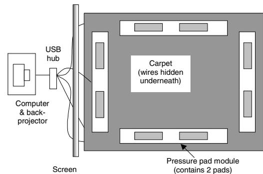
Figure 1: layout of the second prototype ( 8 sensor pads)
