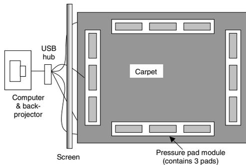
**Figure 3: layout of the third prototype (12 sensor pads)**
