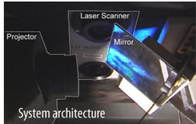
Figure 2. The Scanner, Projector and Mirror setup
