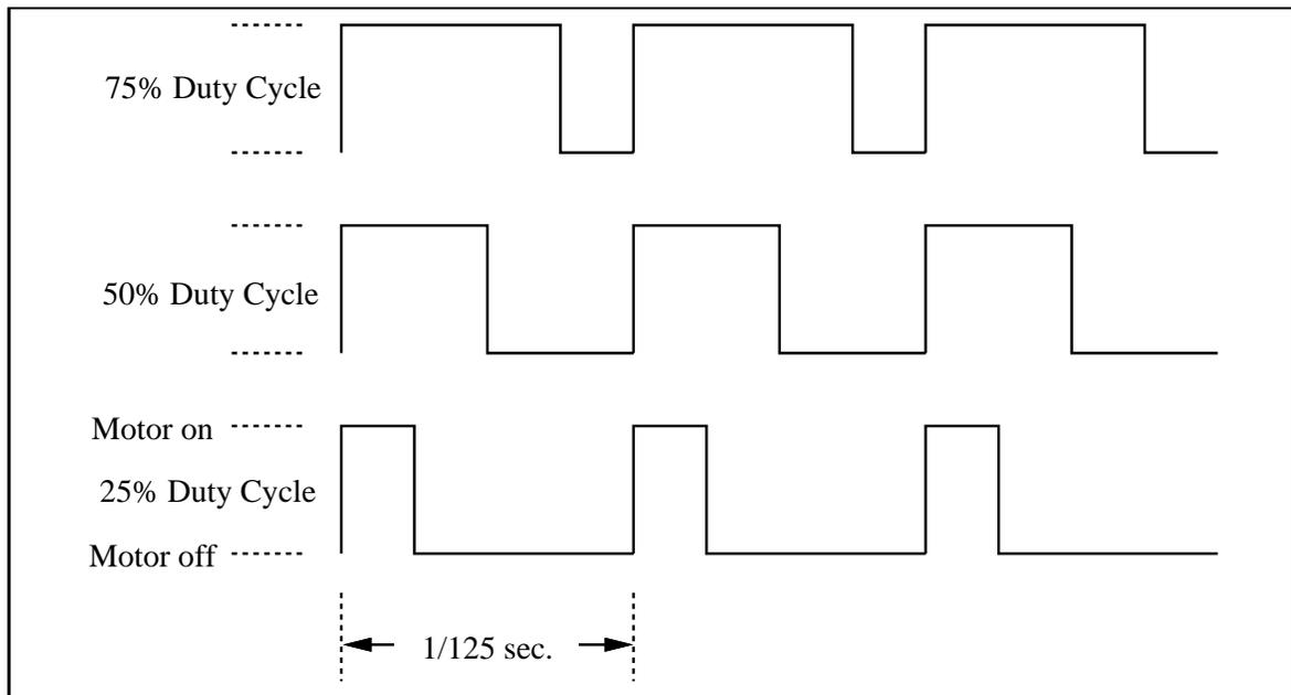
Figure 2.3: Example of Several Pulse Width Modulation Waveforms
