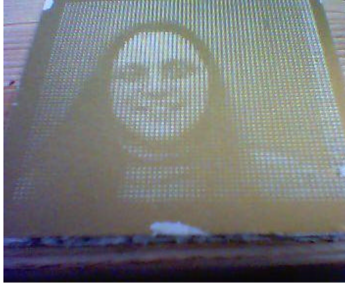
Fig 7. Natasha's portrait using a linear Intensity->Depth mapping function.
