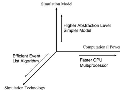
Fig. 1. Different ways to speed up simulation
