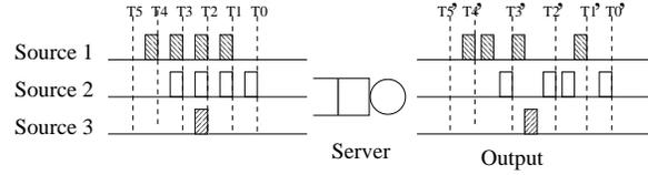
Fig. 3. Dynamics of a FIFO packet multiplexer
