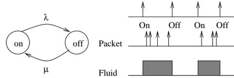
Fig. 2. The on-off fluid source and packet source
